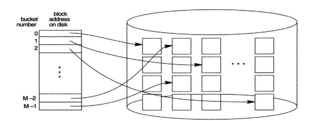
The hashing scheme is called **static hashing** if a fixed number of buckets is allocated. A major drawback of static hashing is that the number of buckets must be chosen large enough that can handle large files. That is, it is difficult to expand or shrink the file dynamically.
